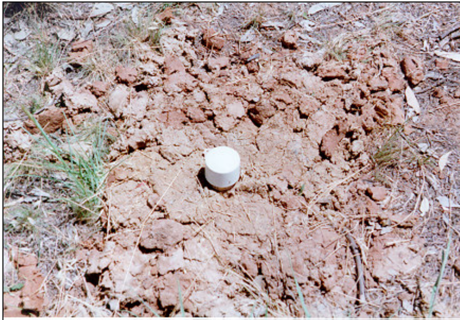
Figure 2 Four bores have been installed in the Reserve to monitor water table levels
