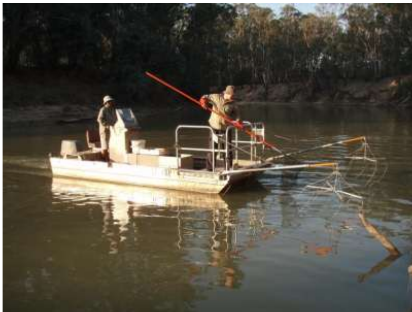
Figure 2. Collecting fish using the electrofishing boat.
