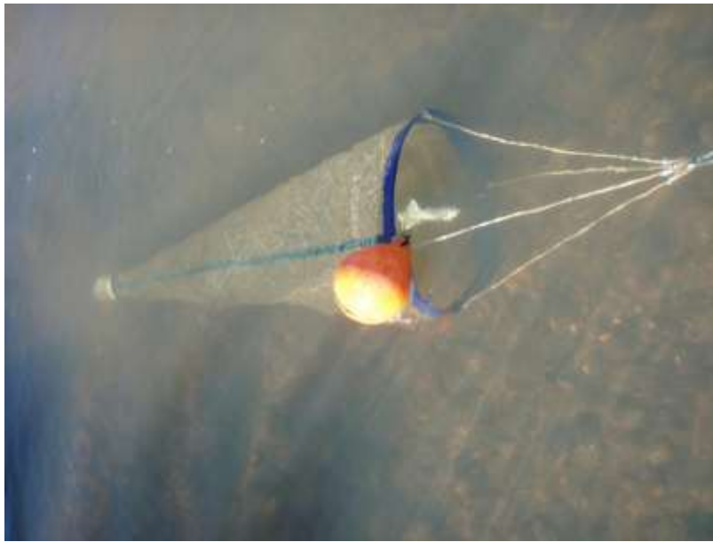
Figure 3. Drift net used to collect drifting fish eggs and larvae.
