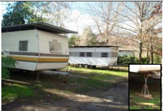
j. Mobile on-site van; inset shows “stacker-jack” used to level the caravan (North East CMA)
