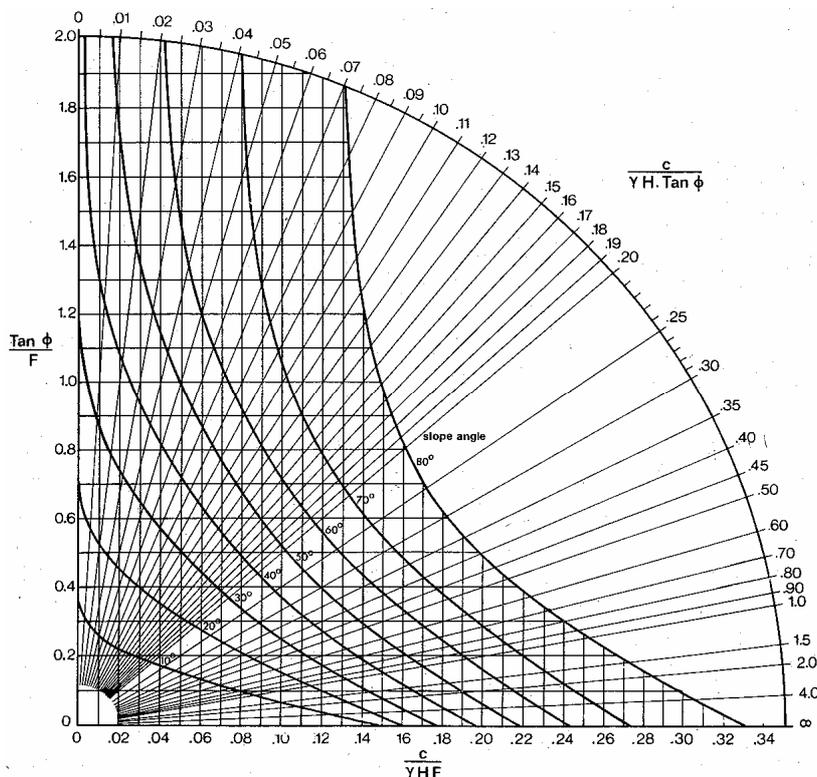
Figure 4.3: Circular failure chart (Hoek and Bray, 1981 p. 238)
