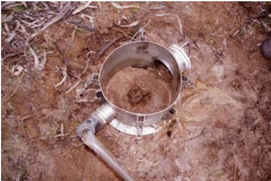
**Figure 4.2: Scour hole produced during 40 minute test.**
