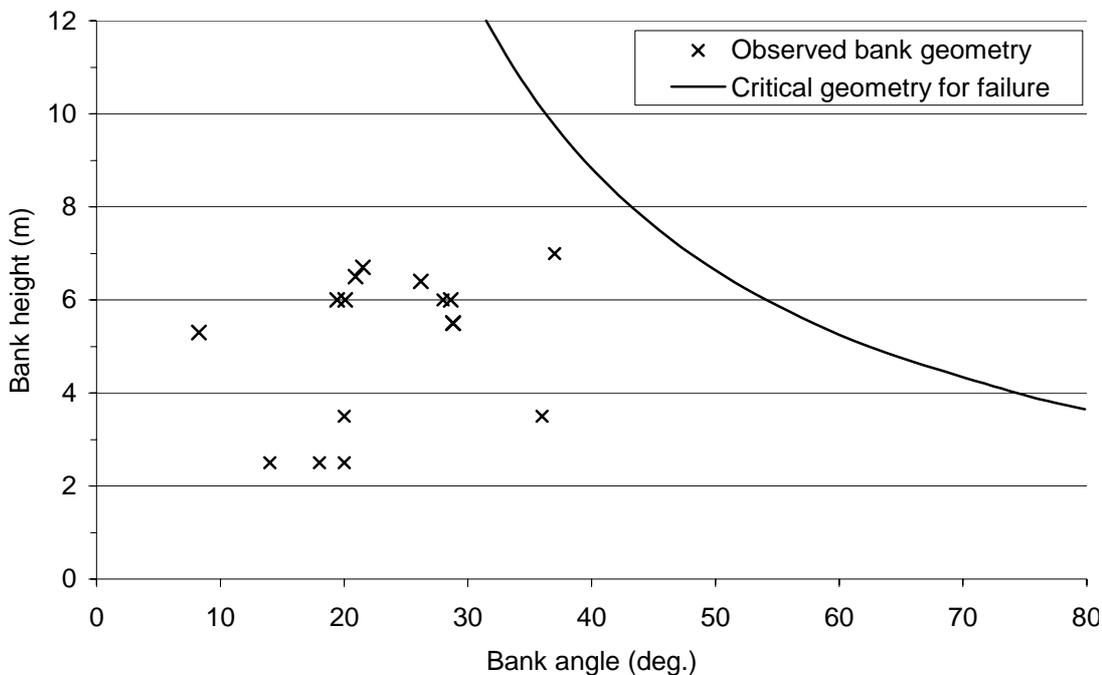
Figure 4.4: Bank geometry of the Deep Creek system compared to critical conditions.
