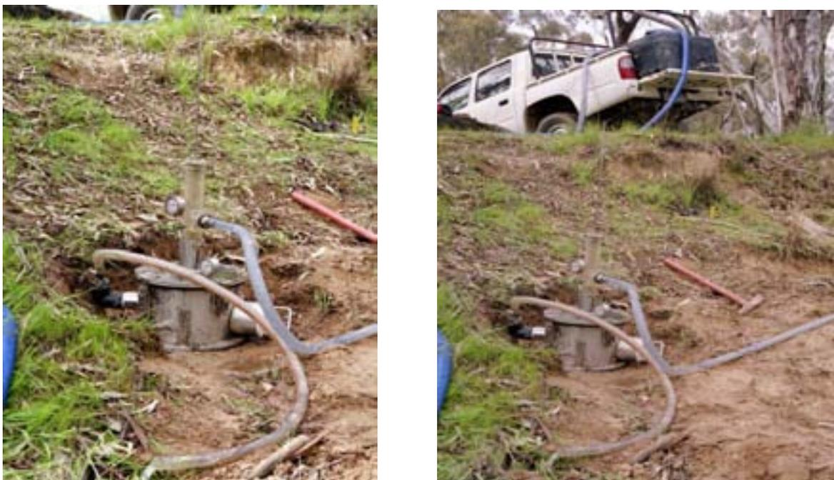
Figure 4.1: The submerged hydraulic jet device in situ.
