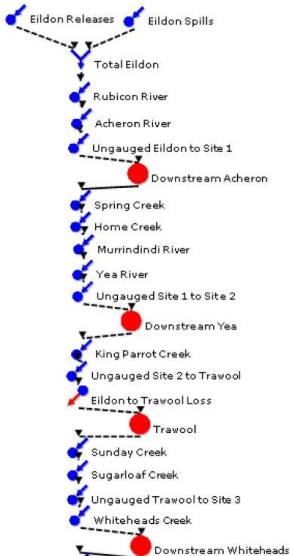
Figure 7: Daily timestep Source model of the main stem of the Goulburn River
