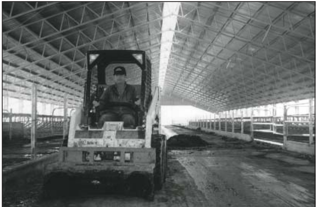
Figure 22: The bobcat with an old tyre used for scraping the bays prior to flood washing.
