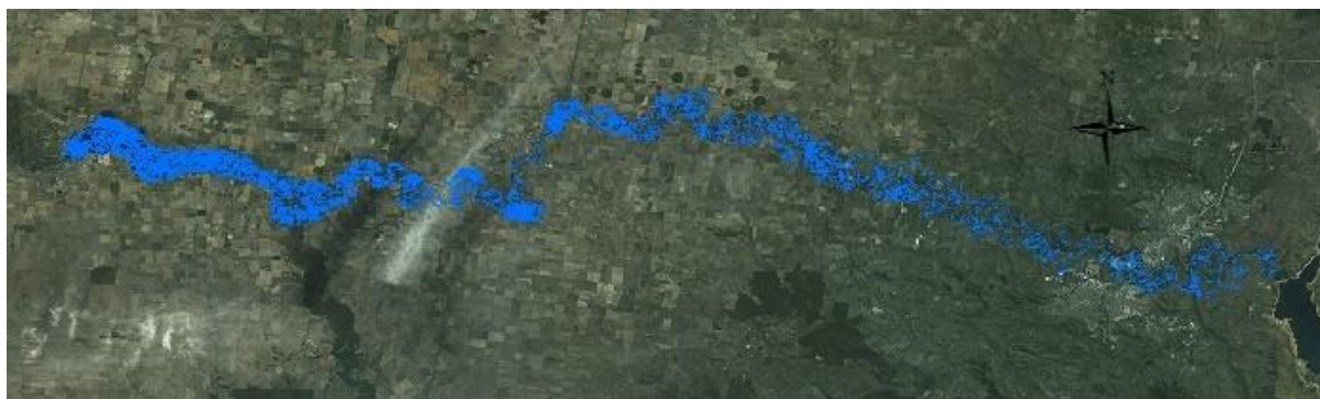
Figure 1: Extent of inundation for the maximum flow provided (50,000 ML/d) in the Hume to Yarrawonga reach
