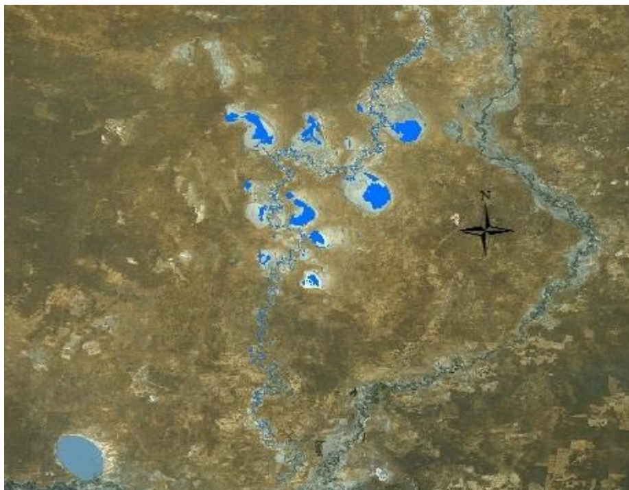
Figure 9: Extent of inundation for the maximum flow provided (17,000 ML/d at Weir 32) in the Lower Darling Zone 2
