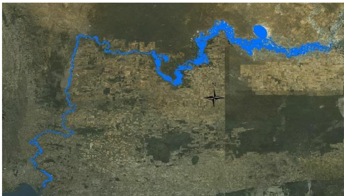
Figure 15: Extent of inundation for the maximum flow provided (125,000 ML/d) in the South Australia reach
