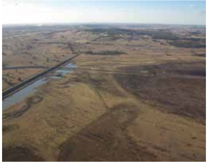
The extended drought has dried Lake Mokoan before it has been decommissioned as a water storage! The only water remaining in late 2008 was in the borrow pits near the wall. The different soil of the original wetlands is clearly visible even though the whole area was covered for most of the time since Lake Mokoan became operational in 1972. Photo: David Pasztaleniec, DSE
