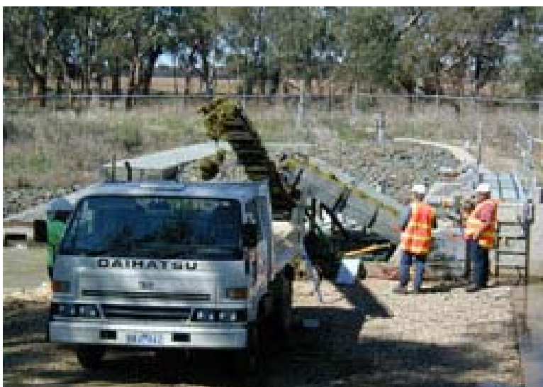
The trial showed the harvester can collect about 2.5 cubic metres of azolla weed per minute of azolla and deliver it to a truck on the adjacent bank.
