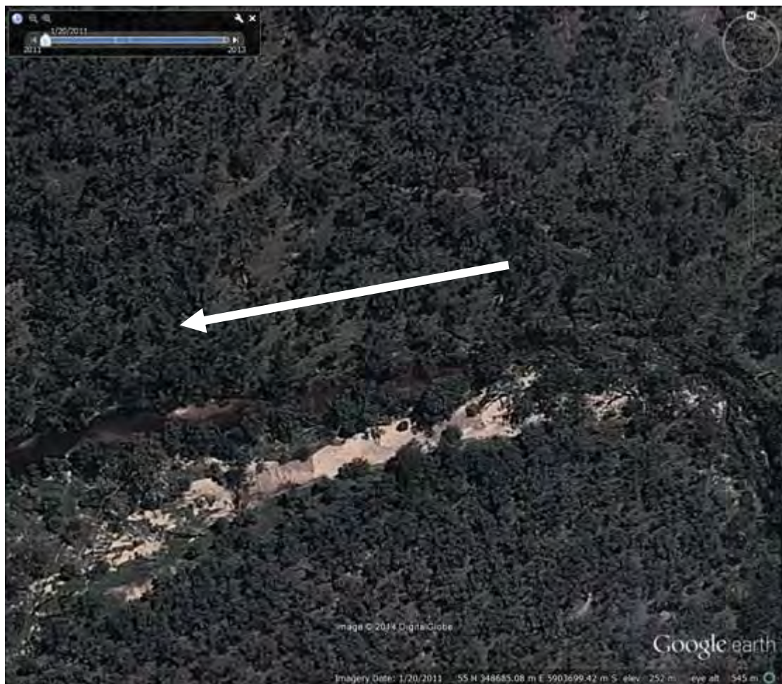
Figure 34 Anabranh infilled with sand by the September 2010 flood in Reach 4 of Hughes Creek.
