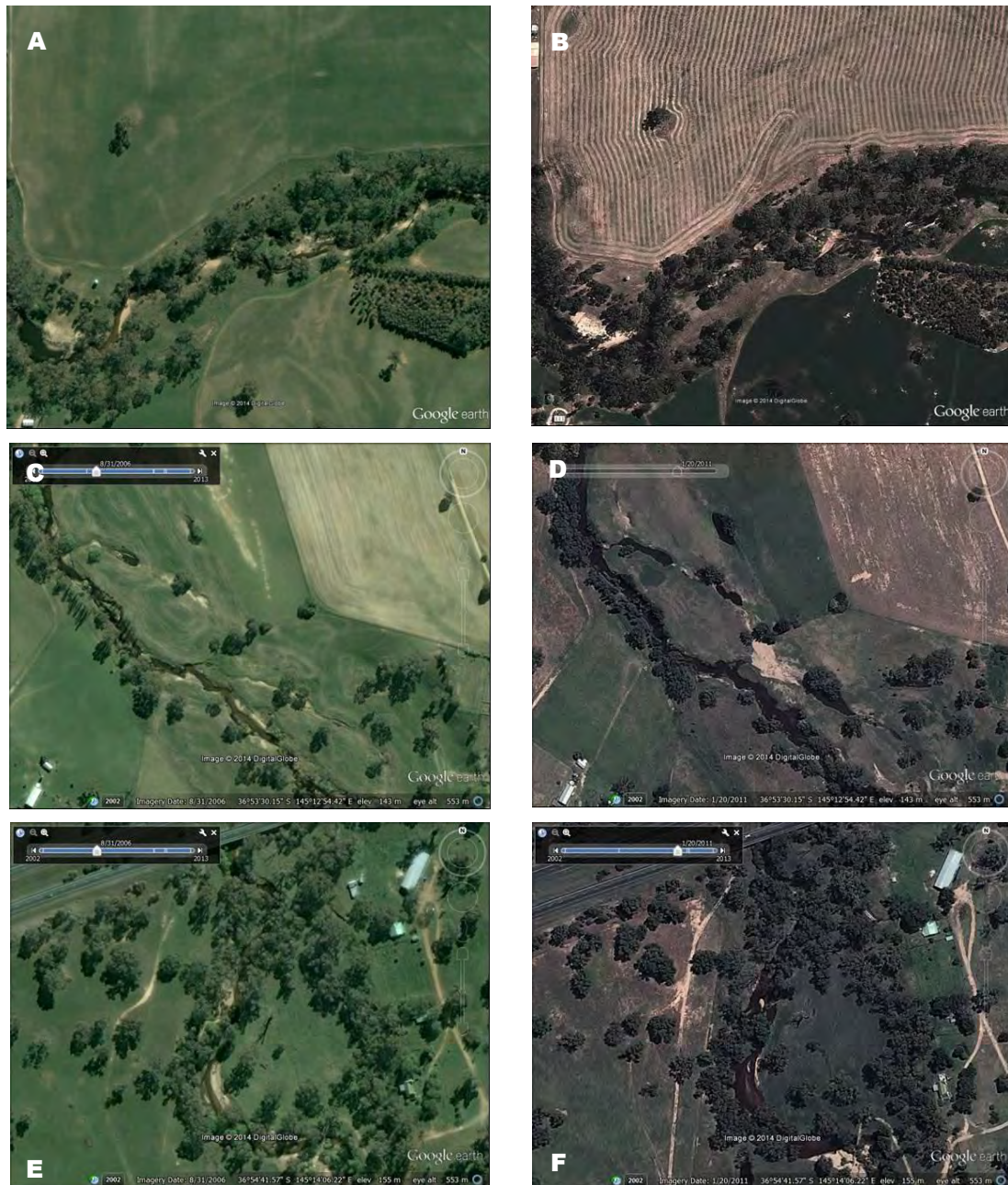
Figure 33 Channel changes produced by the September 2010 flood in Reach 2 of Hughes Creek. Photos on left taken on 31 August 2006 and photos on right, 20 January 2011. (A) and (B) upstream of Goulburn Valley Highway; (C) and (D) at Avenel; and (E) and (F) upstream of Hume Freeway.
